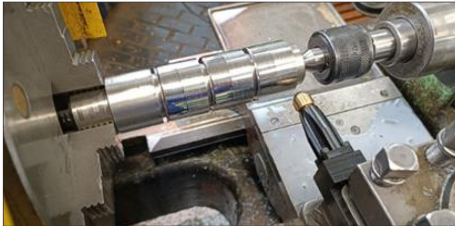
Figure 3. View of a hydrostatic burnishing tool and shaft on a lathe
