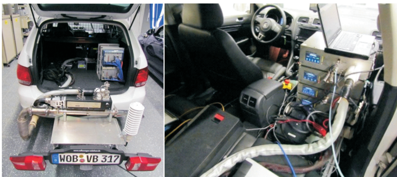
Fig. 22: Validator equipped with PEMS
