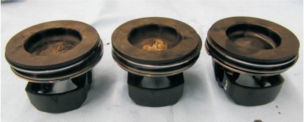
Fig. 6. Steel pistons with coking after engine testing
