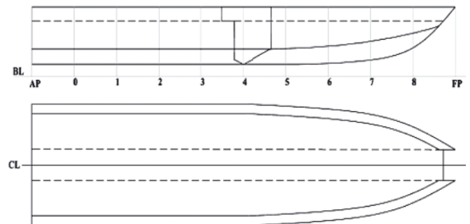
Fig. 6. Catamaran model hull lines drawing
