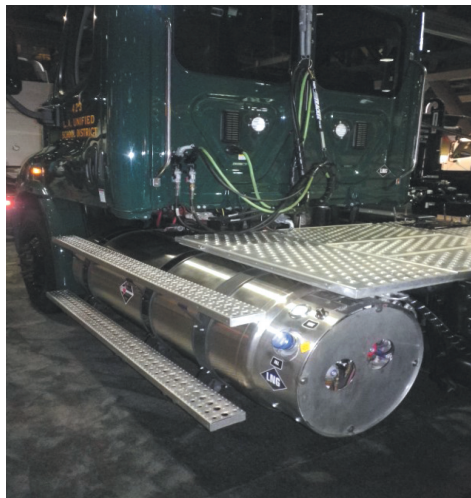
Fig. 5. Truck vehicle with LNG fuel [own materials]
