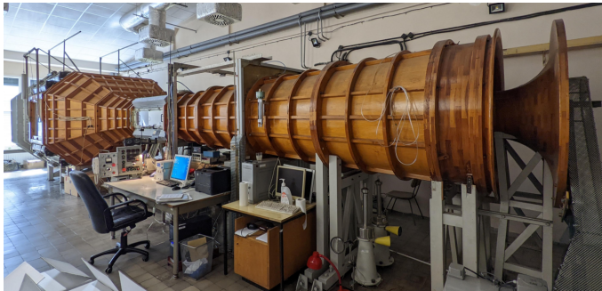
Fig. 4. Wind tunnel at the Calibration Laboratory for Ventilation Measuring Instruments
