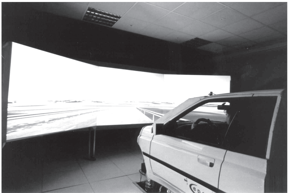
Figure 1a, Figure 1b. The experimental device: the driving simulator (PAVCAS: Poste d'Analyse de la Vigilance en Conduite Automobile Simulée [vigilance analysis driving simulator]).
