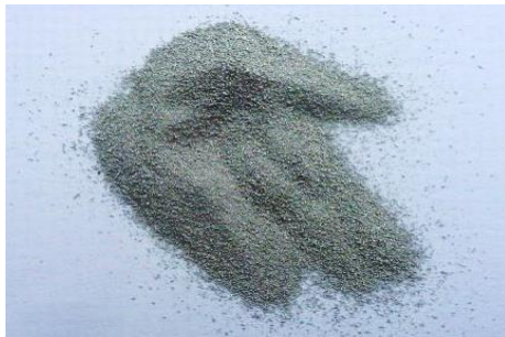
Fig. 4 Powder obtained after spraying. Fraction 50 \mu\text{m} \leq d < 160 \mu\text{m} .
