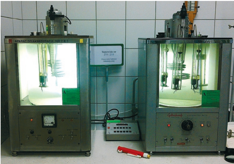
Fig. 1. The workstation used to measure the kinematic viscosity; Department of Performance Testing, Oil and Gas Institute in Kraków Source: Own elaboration
