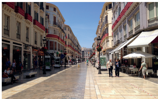
Fig. 2. Shared zone. The arrangement of street furniture (lighting, rubbish bins, tables) in a way that does not reduce the minimum width of pedestrian traffic space. Spain. Photo: W. Tracz
