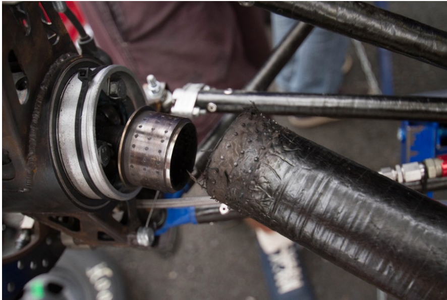
Fig. 12. Composite drive shaft failure
