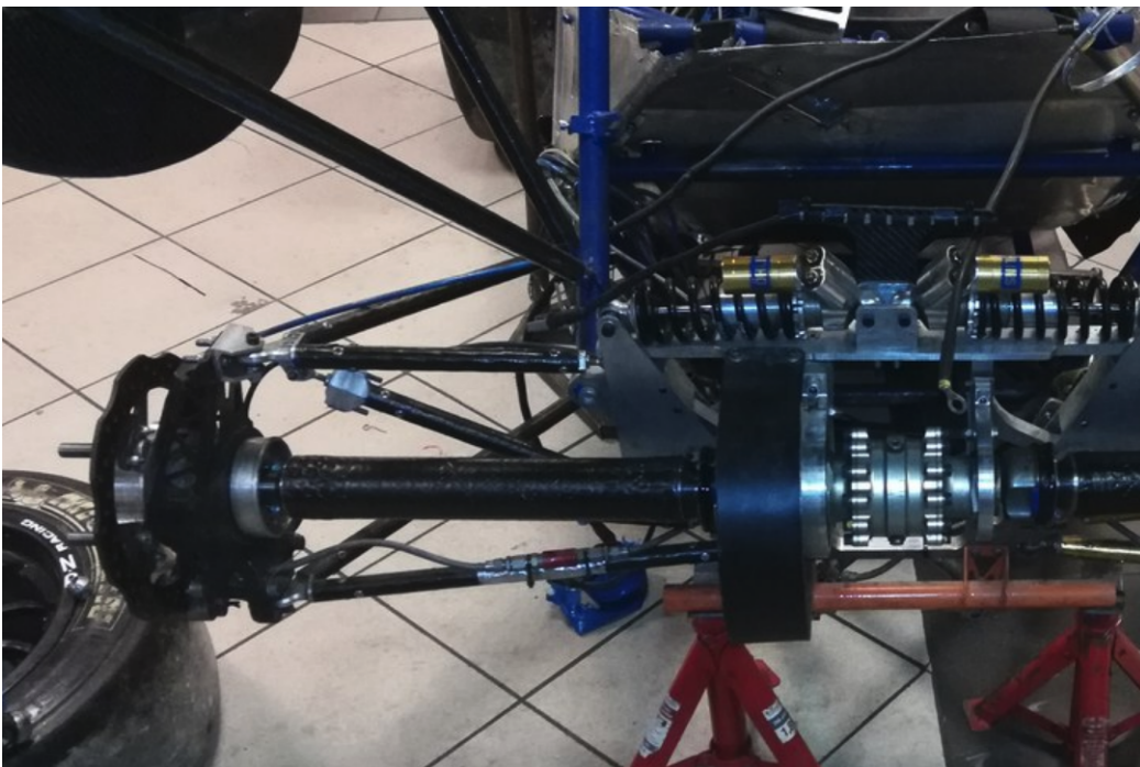
Fig. 14. Formula student car with new design composite drive shafts installed
