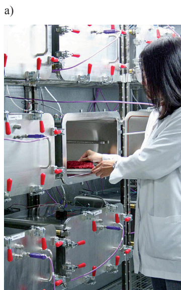
Fig. 2. VOC emission testing chamber: a) 0.053 m 3 , b) approx. 50 m 3 [https://www.mastest.com/voc-testing]
