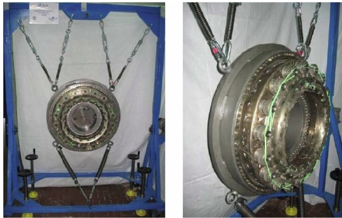
Fig. 3. Experimental set-up: details on boundary conditions
