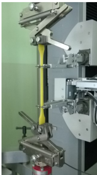
Fig. 2. The uniaxial tension test of elastomer sample
