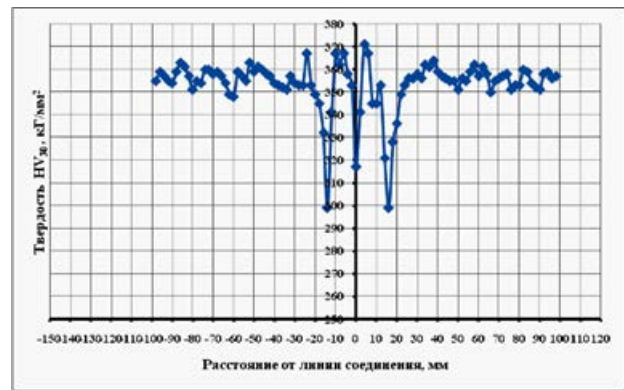
Fig. 8. Diagram of distribution of hardness HV30 in welded joint of rails: R 260 (left), R 350HT(right)
