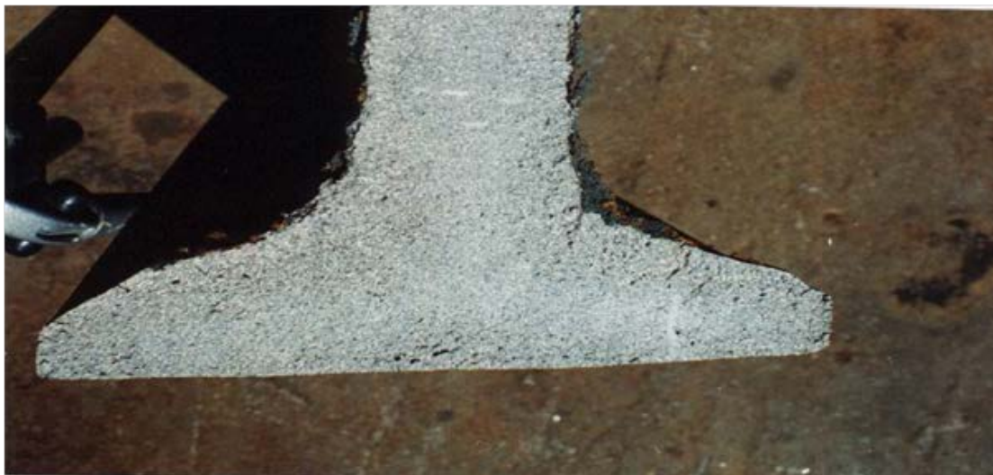
Fig. 4. Dull spots on the fractured surface of the welded joint
