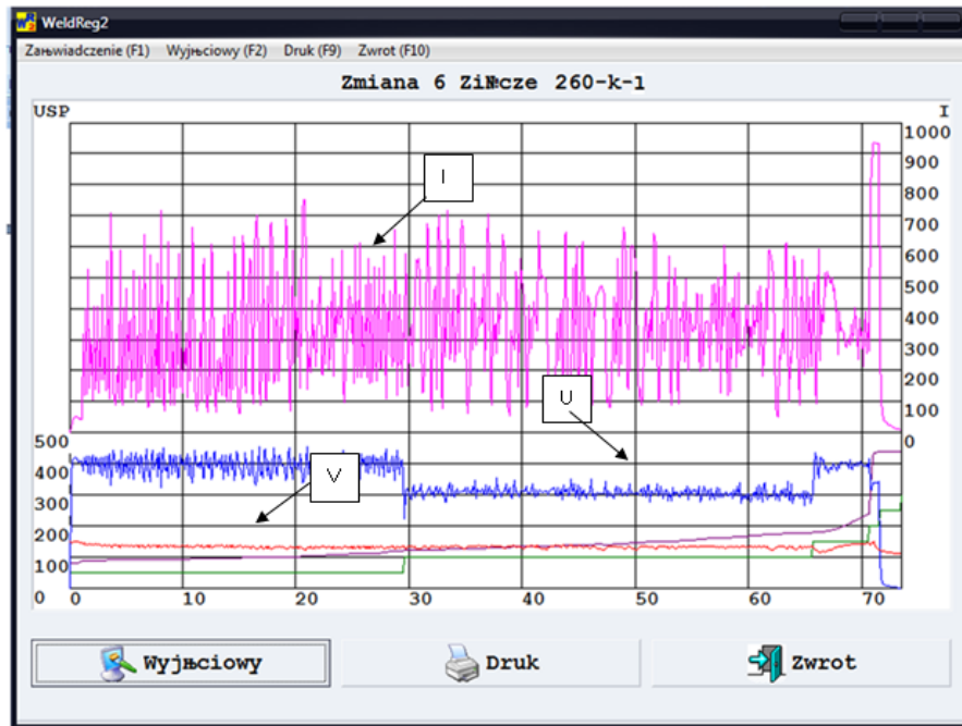
Fig. 5. Program of changing main welding parameters
