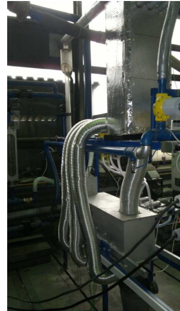
Fig. 2. The way of the air supplying into three independent sectors of the fluidised bed
