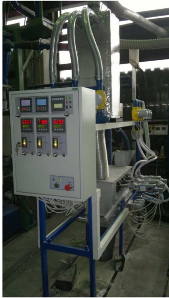
Fig. 1. View of the experimental stand for the thermal reclamation – control panel
