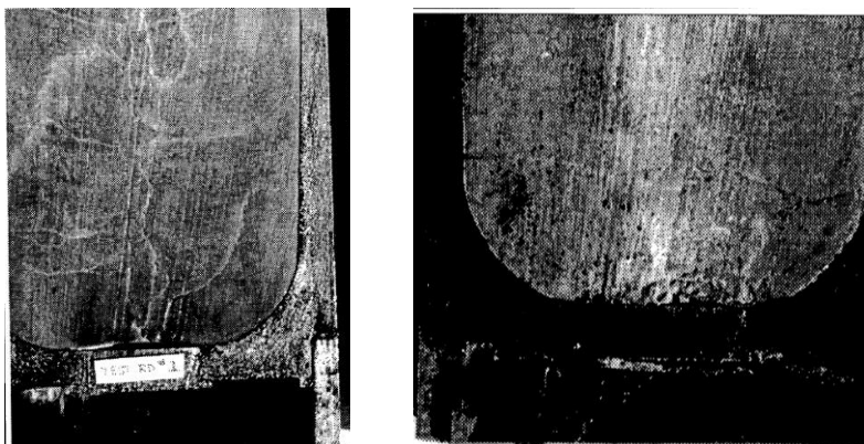
Fig. 5. Photographs cross sectioned 155 mm Comp-B cast projectiles with observable cracks (left) and porosity (right) in the explosive fill [16]
