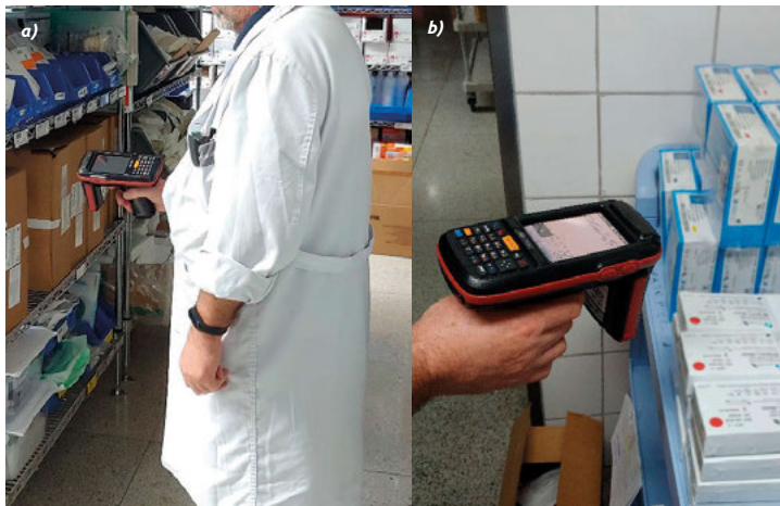
Figure 2 Handheld UHF RFID gun reader: a) an example of the body position of the operator scanning wares marked by RFID tags, b) an example of the manual reading of tagged object Source: Authors' collection.
