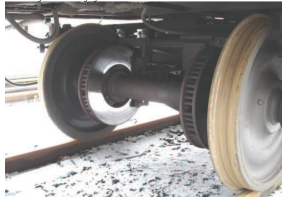
Fig. 1. View of two friction set mounted on axle passenger car
