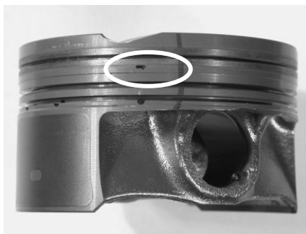
Fig. 2. Shrinkage cavity on the connection place of ring with the piston
