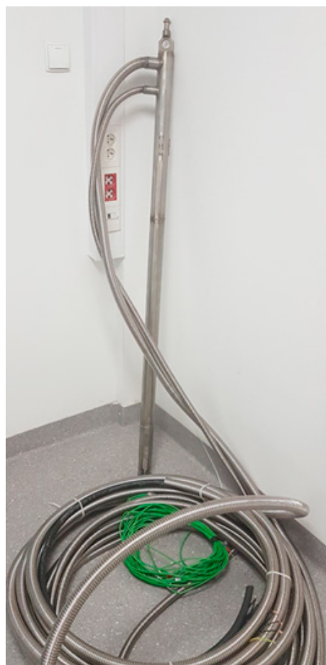
Fot. 2. Termostatyczna sonda badawcza ISTHAR (fot. NCBJ) Photo 2. The ISTHAR thermostatic research rig (photo NCBJ)
