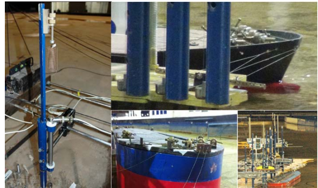
Figure 5. Forces measurement system in the scale model of Sao Marcos Bay – CTH – University of Sao Paulo.
