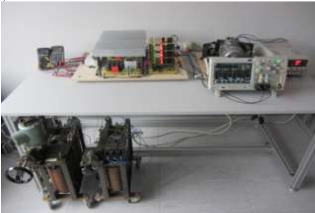
Fig. 2. Two-phase current decay circuit : a) schematic diagram with b) current-voltage measurement ratio 0,4 V - 1 A and c) general view
