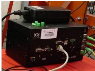
Fig. 5. FBG monitoring system
