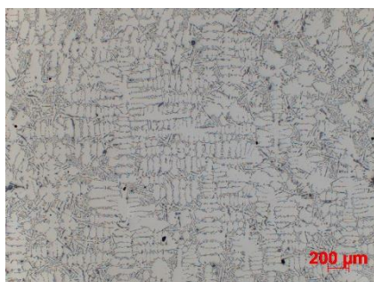
Fig. 4. The dispersion of dendritic structure in the central part of casting, 50x magnification: ablation mould
