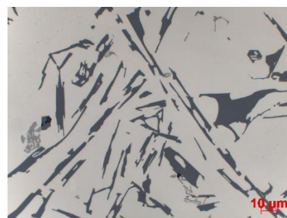
Fig. 7. The morphology of eutectic silicon in the central part of casting, 1000x magnification; ablation mould
