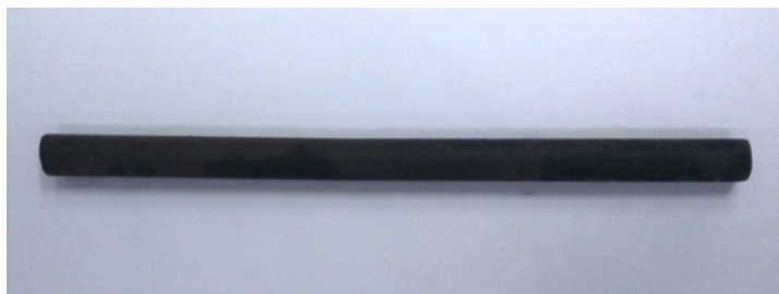
Fig. 1. Appearance of ROCKSPLITTER TM device after burning out of its pyrotechnical mixture.
