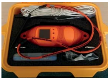
Fig. 11. Sonic sounder for measuring sound speed
