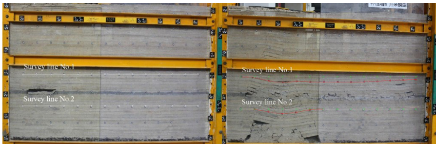
Fig. 4. The fractures after mining of the lower coal seam has been completed. The fractures above in the image are shown by the yellow lines
