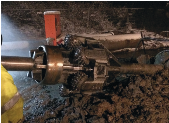
Fig. 1. Roll reamer (Hole Opener) before tripping to the borehole [collection of J. Janicki]
