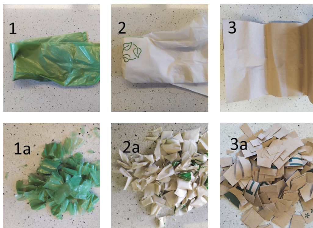
Fig. 1. Tested materials 1–1a. Oxy, 2–2a. Corn, 3–3a. Pap before and after shredding (photo: Biernacki, M.)
