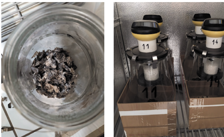
Fig. 3. Sample in glass container (left), and OxiTop system in thermostatic cabinet (right) (photo: Biernacki. M.)
