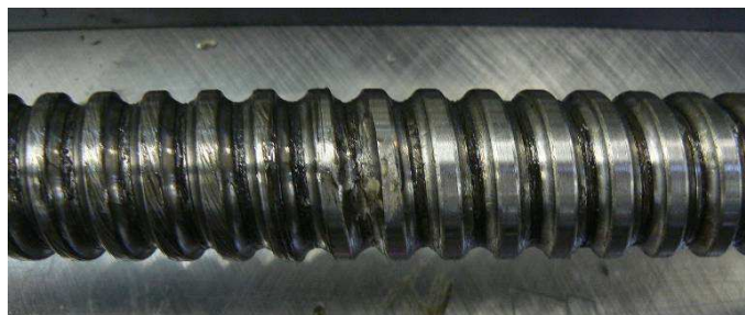
Fig. 12. Prepared damage on the shaft
