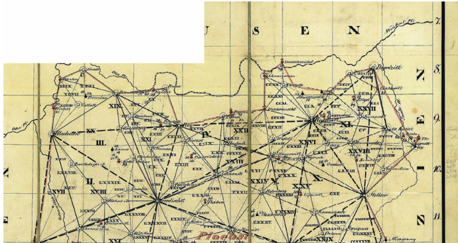
Fig. 6 – A part of the sketch of the trigonometric network in the territory of Ostrava (surveyor Ploebst).
