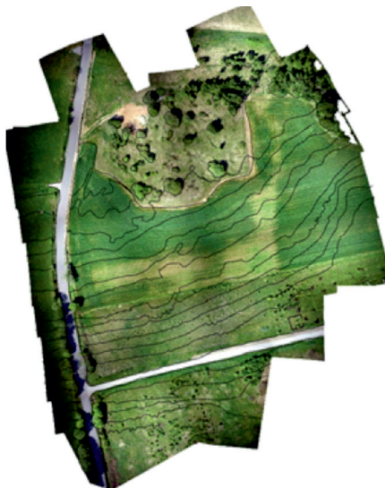
Fig. 4. Topographic elements vectorized according to the results of the OBIA classification on the orthophotomap
