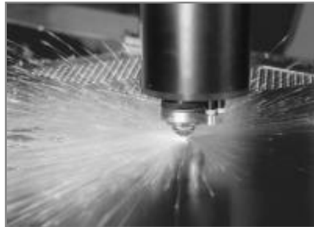
Fig. 3. Cutting bores with a laser cutter
