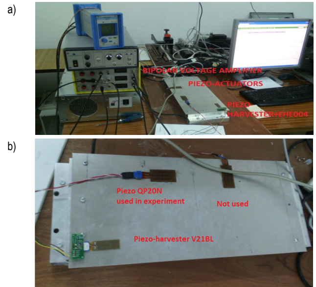
Fig. 8. a) The photo of the laboratory stand, b) the photo of a smart plate with piezo-elements (actuators QP10N and harvester V21BL) located on their top surface
