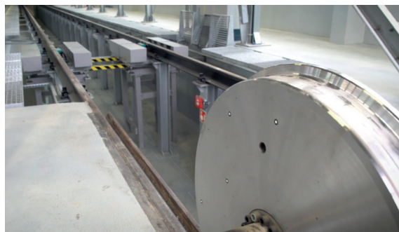
Fig. 6. Integrated device for laser measuring of flat area on wheels and stickers on the wheels [own study]
