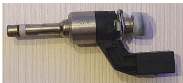
Fig. 1. View of the fuel injector and external deposits in the area of the fuel outlet holes – VW EA111 BLG test engine
