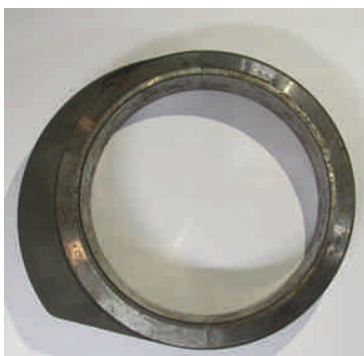
Fig. 5. The image the fuel cam of the inspected engine
