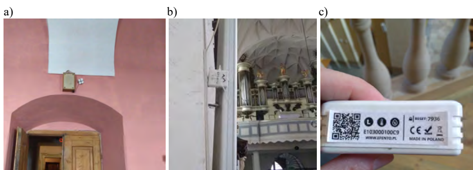
Fig. 4. Mounted sensors for measuring the temperature and humidity of the interior air a) in a church in Wigry over the entrance b) in the St. Andrew the Apostle's church in Barczewo c) in St. Anna's church in Barczewo d) general view of the mounted sensors
