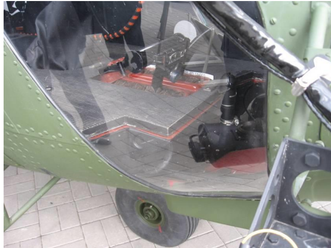
Fig. 11. Polish solution of light armor for the Sokół helicopter. Aramid laminate Lim M1 with corundum ceramics SiC Source: [Gula 1992].
