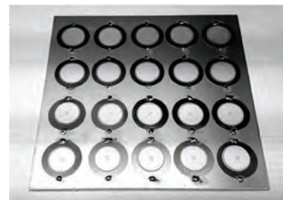
Fig. 4. PZT converter, consisting of 20 PZT/brass disk transducers fixed to a common copper surface.
