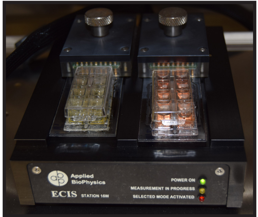
FIG. 3. Nickel matrices with A-375 melanoma cell culture (left) in the ECIS ® measuring station.
