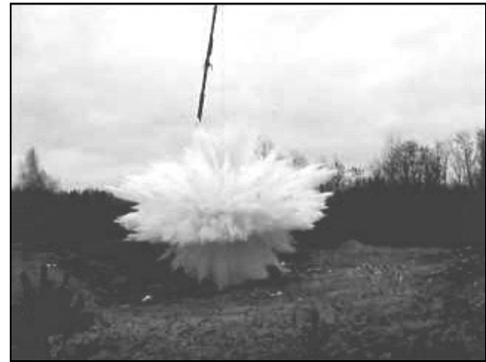
Fig.2. The formation of a water aerosol cloud (cylindrical configuration) : A – 40 ms, B – 80 ms and C – 160 ms after beginning of explosion
