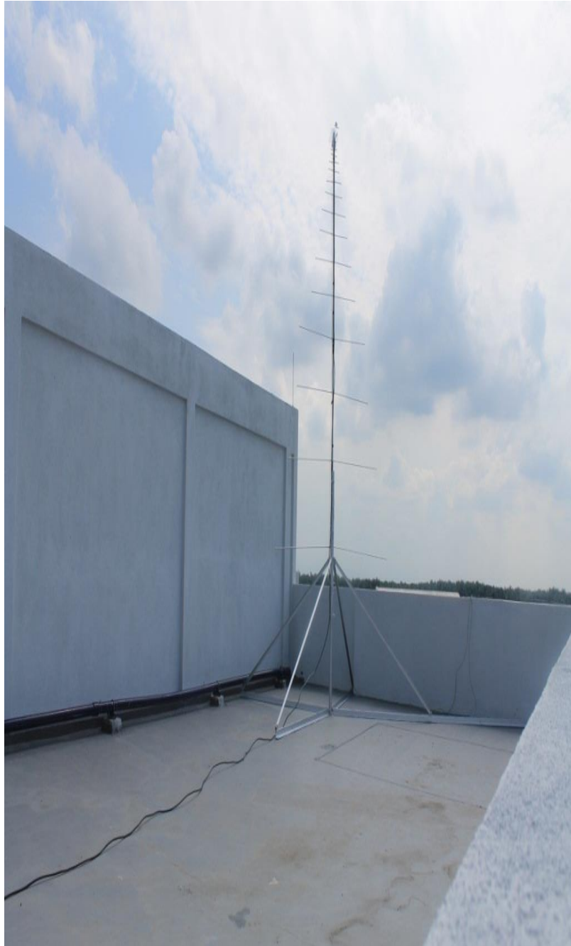
Figure 9. Logarithmic Periodic Dipole Antenna at the National Space Centre, Banting Selangor, Malaysia.
