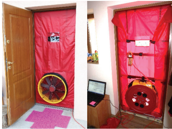
Fig. 2. An installed system for leak testing using the Blower Door method - a view from the outside and from the inside of the building
