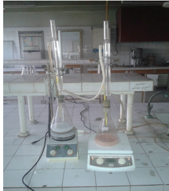
Figure 1: Photograph of the modified Chapelle test set-up.
