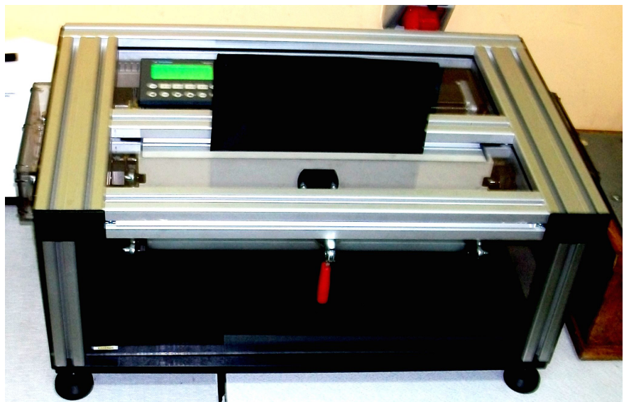
Figure 1. Test stand for fatigue-test of inserts for bullet-proof vests.
