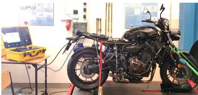
Fig. 5. Picture of the tested motorcycle along with the measuring apparatus on the designated dynamometer
