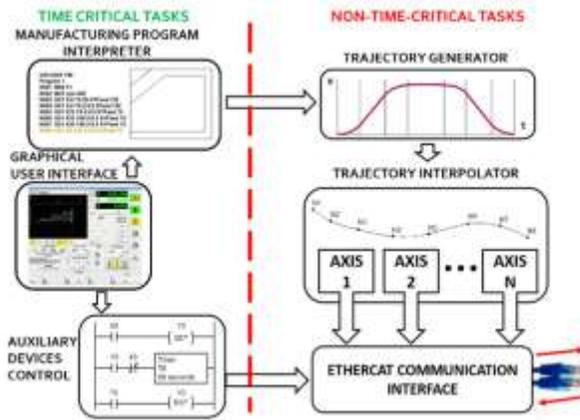
Fig. 2. CNC software modules divided into real-time and non-real time tasks
