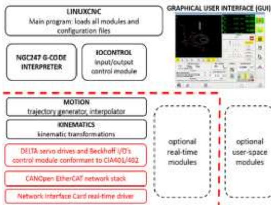
Fig. 3. Structure of LinuxCNC software blocks
