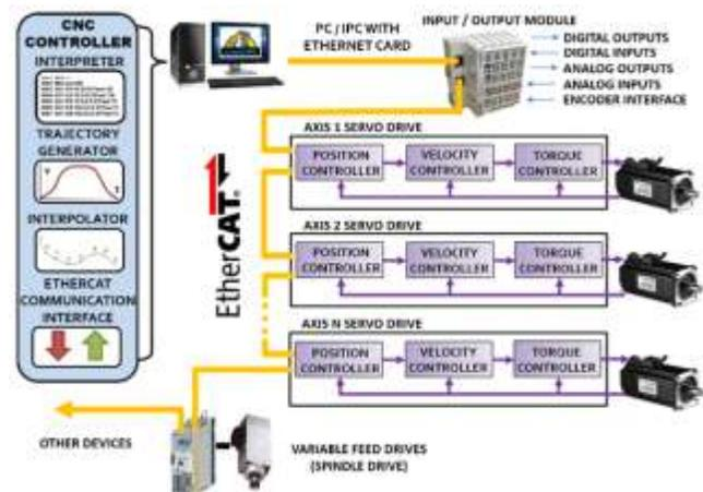
Fig. 1. Block schematic of the CNC control system
