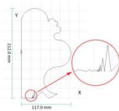
Fig. 9. Toolpath used to test following errors
