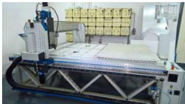
Fig. 8. 3-axis machine with the developed CNC control system
