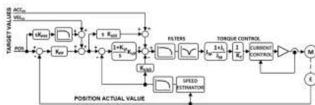
Fig. 6. Position and velocity controller structure of ASD-A2-0721-E servo drive
