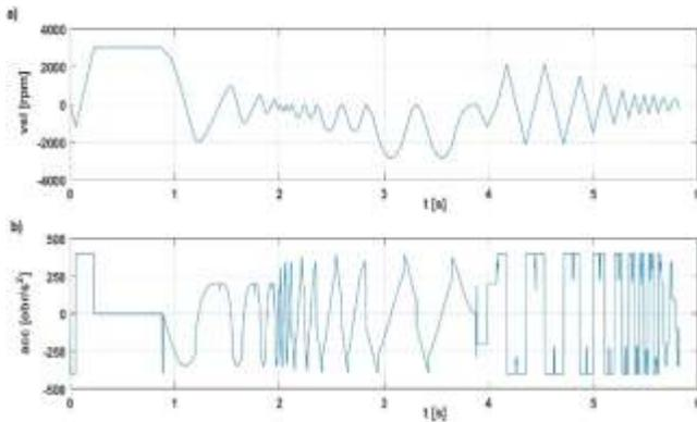
Fig. 10. Velocity (a) and acceleration (b) demand during execution of the test toolpath on the linear motion module
