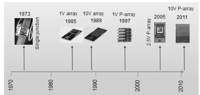
Fig. 1. Milestones of Josephson junction array development at NIST. The "array" refers to zero current bias arrays and the "P-array" refers to programmable arrays using current biased voltage steps
