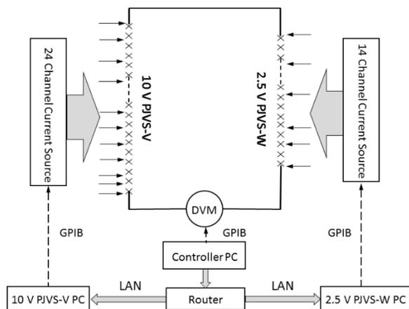
Fig. 4. Setup of an automated comparison between PJVS-W1 and the PJVS-V
