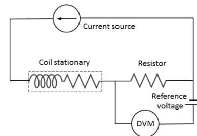
Fig. 3. Voltage measurement in force mode
