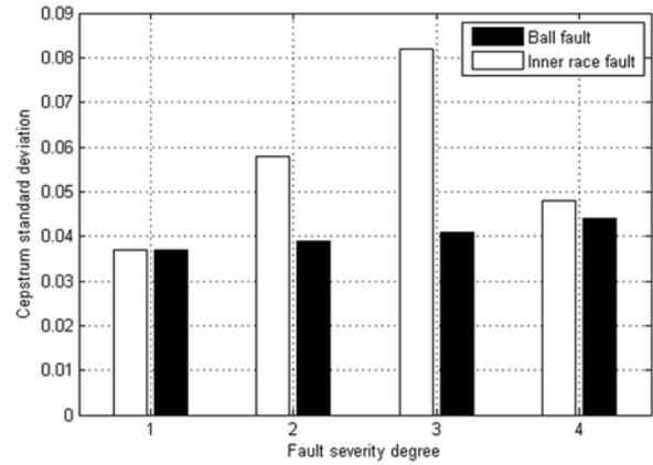
Fig. 6. Standard deviation of cepstra for bearing faults
