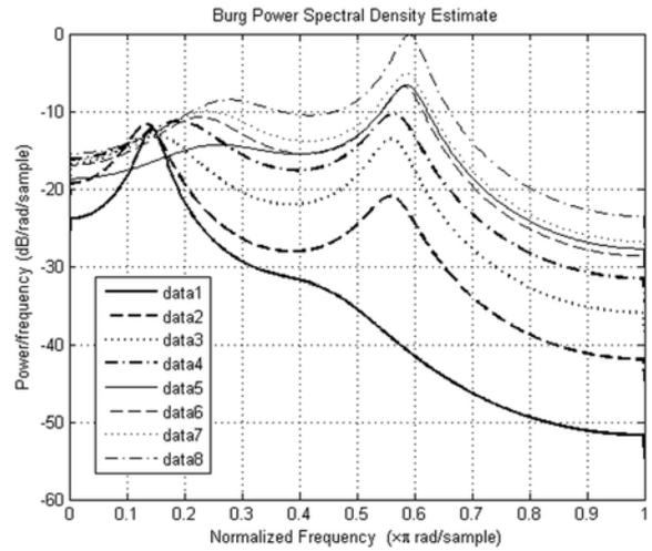
Fig. 1. PSD estimates for artificial motor aging data
