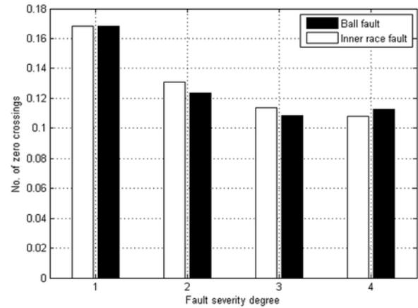
Fig. 8. Number of zero crossings for bearing faults
